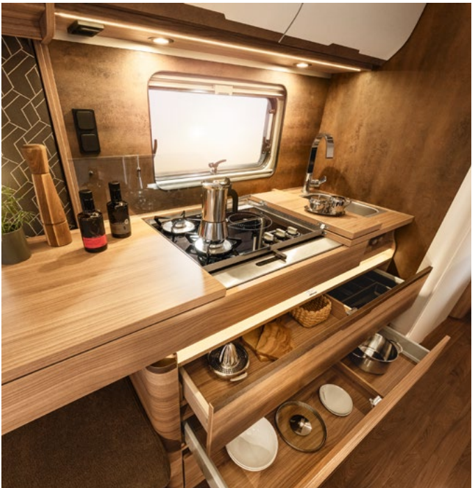
The hybrid hob combines two gas-on-glass burners with an induction hob, opening up a wide range of possibilities for modern cooking comfort. VIVALDI 550 E 2,3
